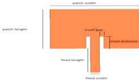
**Fig. 1.** Design of a single MPA
