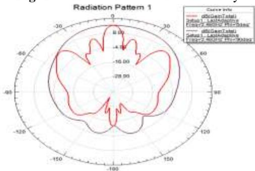
Fig. 16. Radiation pattern of 1x4 array at  $\phi=0^\circ$  (E-plane) &  $90^\circ$  (H-plane)
