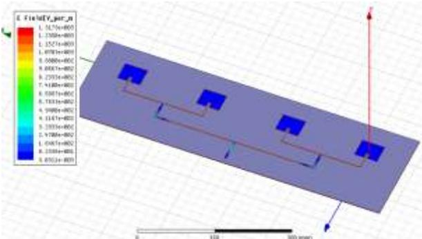
Fig. 14. Current distribution of 1x4 array
