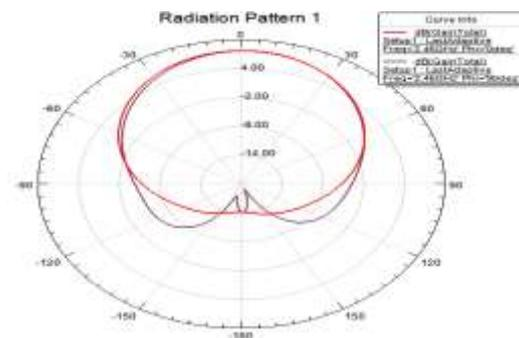
**Fig. 4.** Radiation pattern of single MPA
