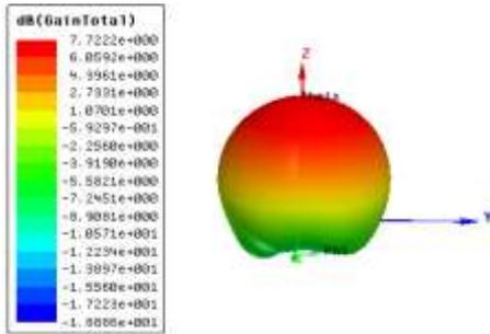
Fig. 5. Polar plot Gain of single MPA
