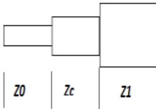
Fig. 7. Impedance matching by quarter wavelength transformer
