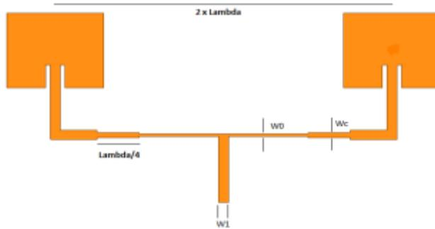
Fig. 8. Design of a 1x2 MPA array
