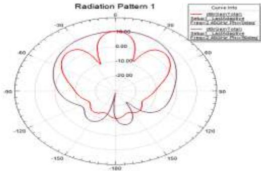
Fig. 11. Radiation pattern of 1x2 array
