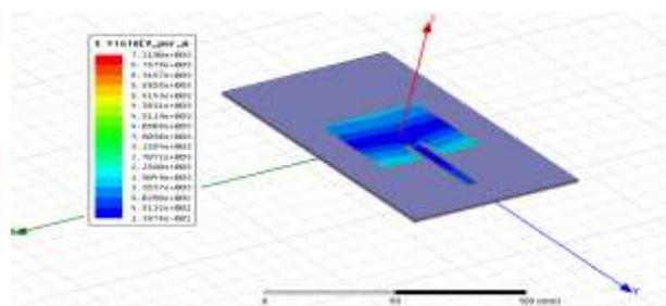
**Fig. 2.** Current distribution of single MPA
